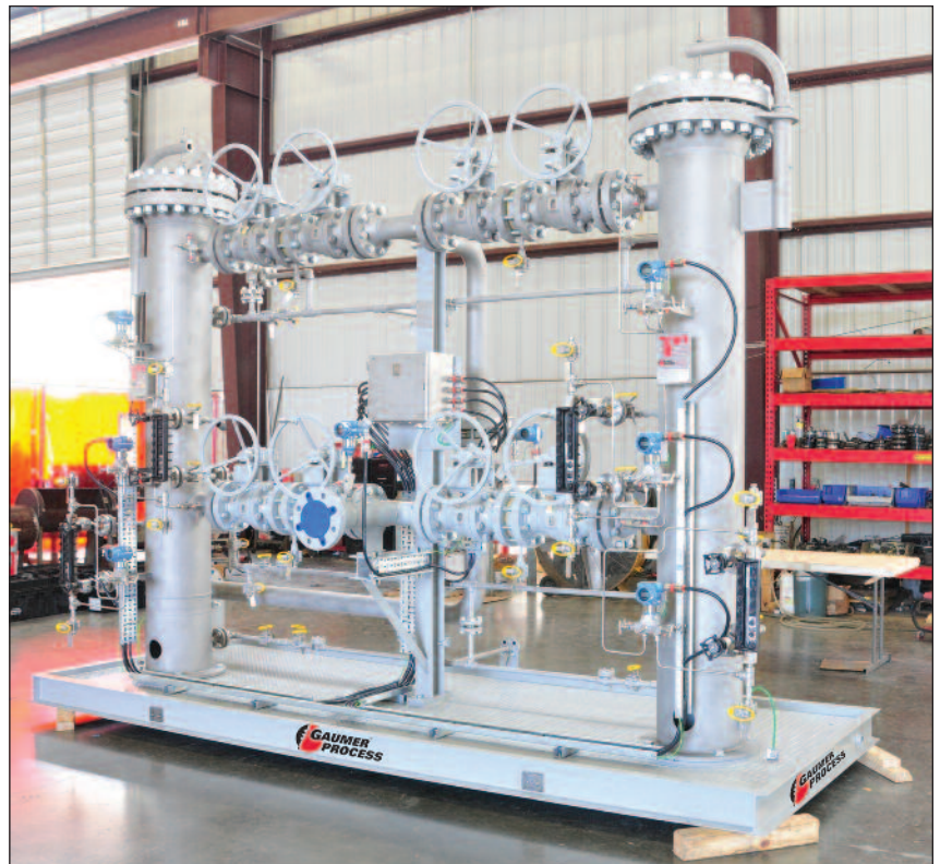
Fuel gas, double block & bleed
